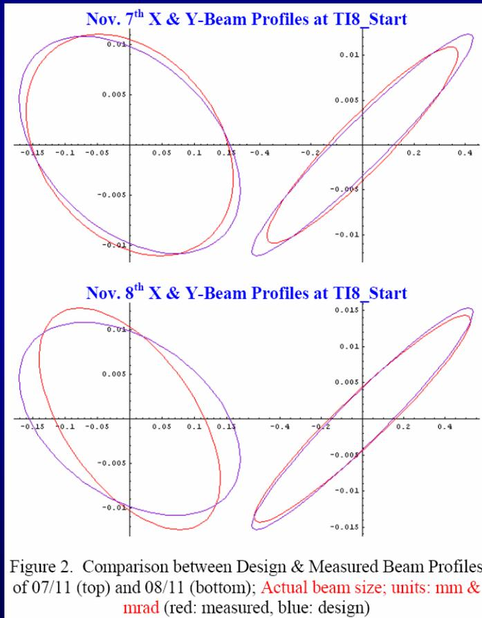
Figure 2. Comparison between Design & Measured Beam Profiles of 07/11 (top) and 08/11 (bottom); Actual beam size; units: mm & mrad (red: measured, blue: design)
