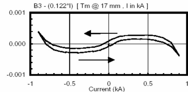
Figure 3 : Field strength of **MCS** corrector : difference between the strength and straight line giving the average to enlighten the hysteresis due to persistent currents.
