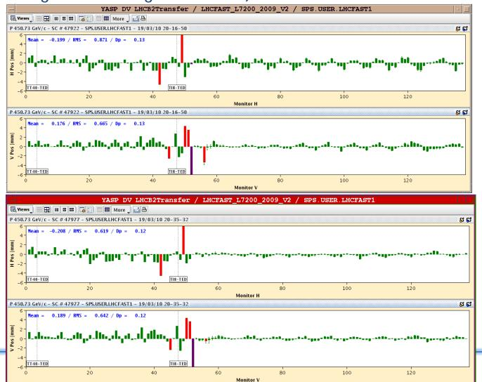
Injection oscillations: B1 corrected by MCIAH.2880 = 9.28 urad (reducing the existing correction)
