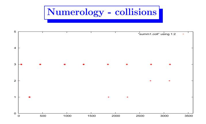
50ns spacing, 12 bunches per train, 108 bunches, maximum head-on: 3
