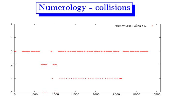
150ns spacing, 8 bunches per train, 424 bunches, maximum head-on: 3
