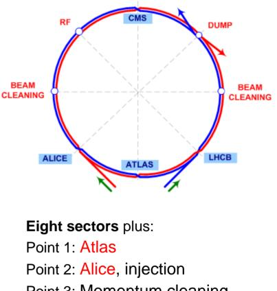
Eight sectors plus: Point 1: Atlas Point 2: Alice, injection Point 3: Momentum cleaning Point 4: RF Point 5: CMS Point 5: CMS Point 6: Beam Dumps Point 7: Betatron cleaning Point 8: LHCb, injection
