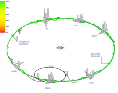
3.3 km of QRL per sector2100 internal welds700 external manual welds
