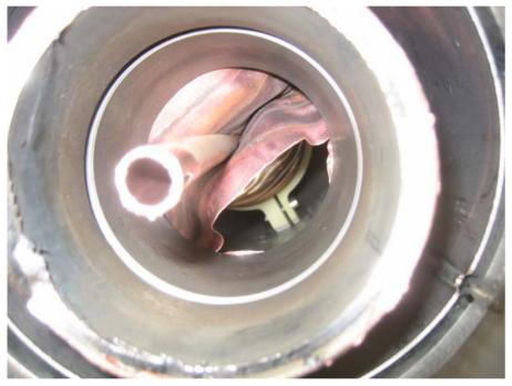
During the pressure test of Sector 8-1 (25<sup>th</sup> November) the heat exchanger tube in the inner triplet failed at 9 bar differential pressure.
