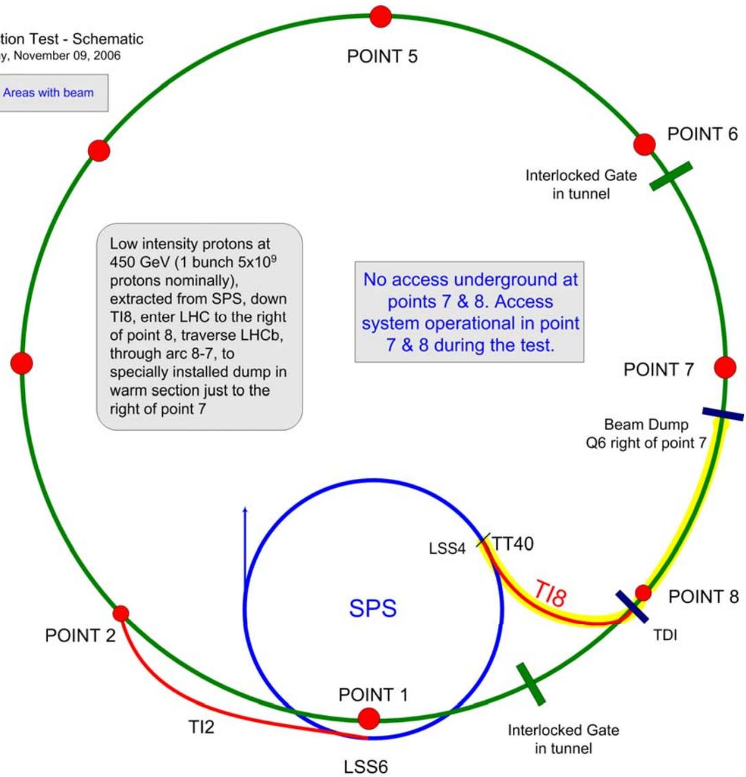
Low intensity protons at 450 GeV (1 bunch  $5 \times 10^9$  protons nominally), extracted from SPS, down T18, enter LHC to the right of point 8, traverse LHCb, through arc 8-7, to specially installed dump in warm section just to the right of point 7
