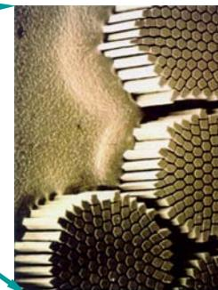
Total superconducting cable required 1200 tonnes which translates to around 7600 km of cable
