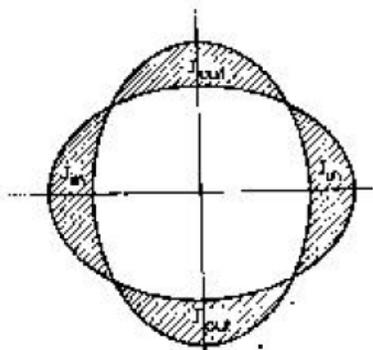
Two intersecting ellipses, rotated by  $90^\circ$ , generate a perfect quadrupole fields
