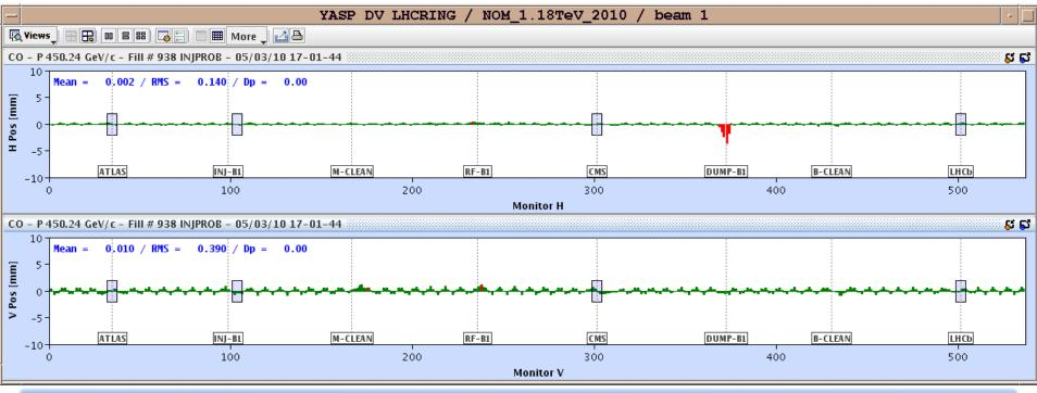
ALICE solenoid : Non-closure in rms: B1 H: 0.24 - V: 0.22 ; B2 H: 0.15 - V: 0.23 Corrected to 0.1 mm rms in both planes, both beams
