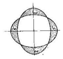
Two intersecting ellipses, rotated by 90°, generate a perfect quadrupole fields
