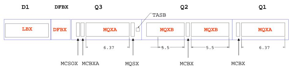
IR 1 and 5, D1 is a normal conducting dipole.
