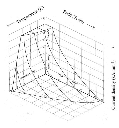
Niobium titanium **NbTi** is the standard 'work horse' of the superconducting magnet business
