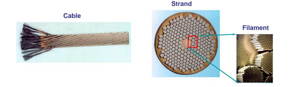
Total superconducting cable required 1200 tonnes which translates to around 7600 km of cable
