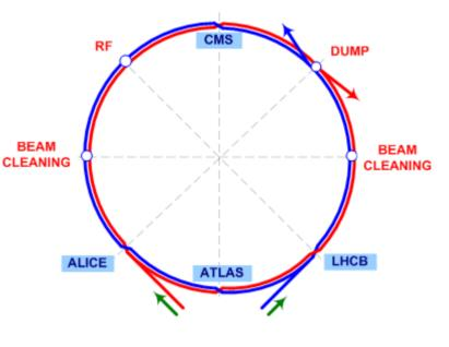
Eight sectors plus: Point 1: Atlas Point 2: Alice, injection Point 3: Momentum cleaning Point 4: RF Point 5: CMS Point 5: CMS Point 6: Beam Dumps Point 7: Betatron cleaning Point 8: LHCb, injection
